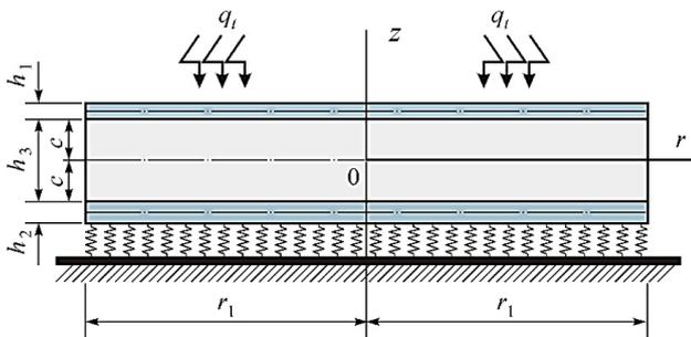
Figure 1: Design model of considered plate
